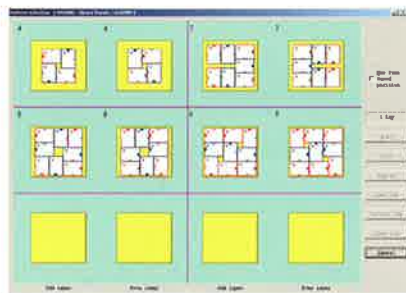
Stacking program is automatically created after selecting a stacking pattern.
