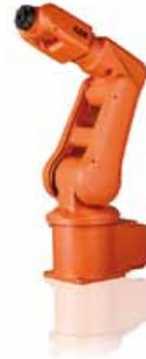
radius, which is enabled by the robot's symmetric architecture, without offset on axis 2. This ensures the robot can be mounted close to other equipment and the slim wrist enables the arm to reach closer to its application.
